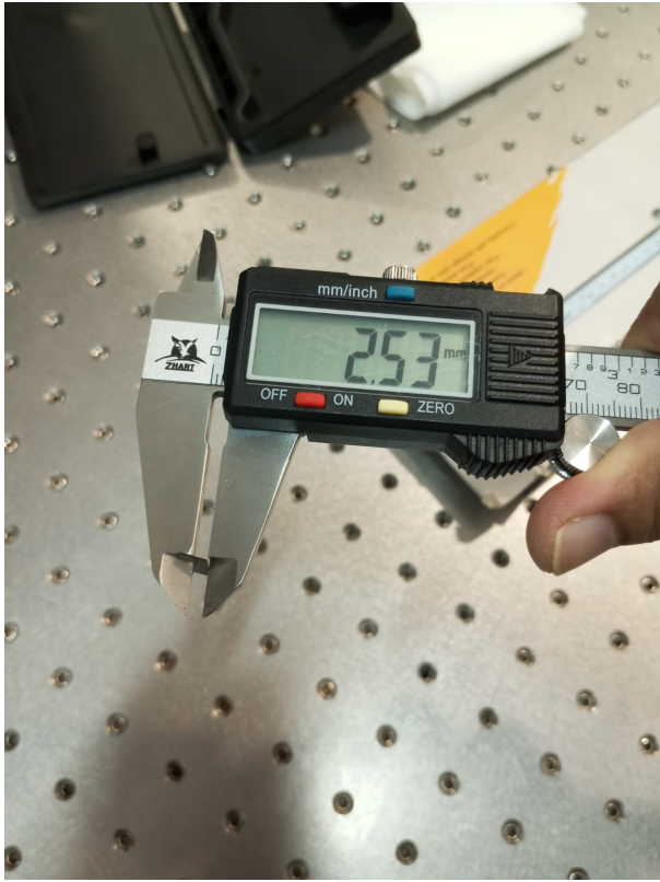
Fig. 2: Post-fabrication dimensional tolerance check using a digital caliper. Measurements confirmed that the prototype satisfied the required tolerance band for CAM fabrication.
